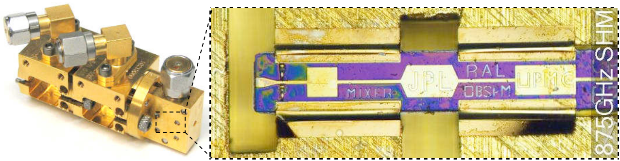
Fig. 6: view of the compact 874 GHz receiver front-end including 200 and 400 GHz doublers, and an 874 GHz sub-harmonic mixer (left hand side). The membrane based biasless chip used for the mixer is shown on the right.
