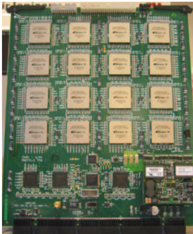
Fig. 2. Photograph of a single correlator digital filter card. There are 32 digital tunable filters implemented in 16 large programmable FPGAs. The filter bandwidth (from 2 GHz to 31.25 MHz), filter shape, and spectral resolution can be selected by the users (see text). The correlator system includes 512 such cards
