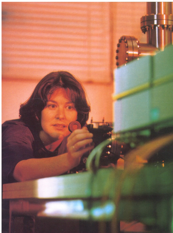
Figure 18: An illustration of laboratory astrophysics: aligning the optics for a laser spectroscopic measurement.
