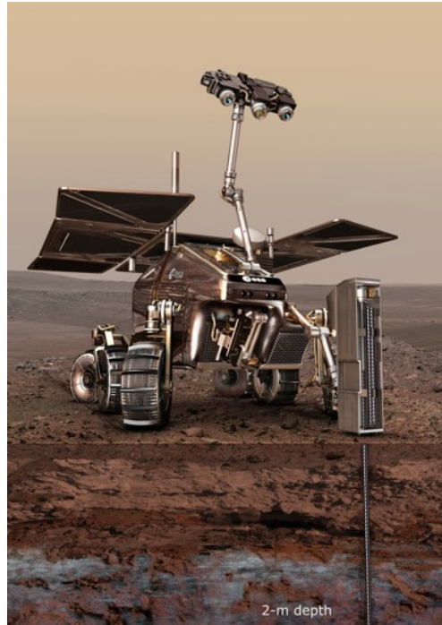
Figure 14: Artist's impression of the ExoMars Rover, which will search for traces of past and present signs of life by drilling into the Martian surface down to a depth of 2 metres. [Image taken from http://www.esa.int/esaMI/Aurora/SEM1NVZKQAD_0.html ]
