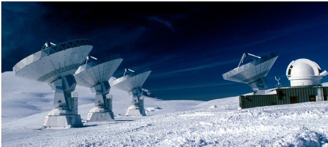
**Experiment at POM2. SIS receiver and autocorrelator providing 39 kHz resolution and 4.53 MHz of total band.**
