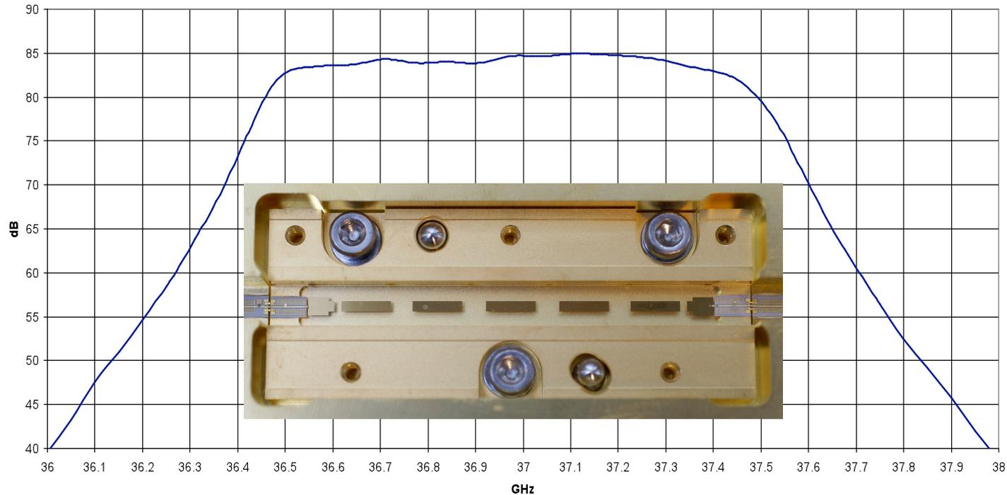
Frequency performances mainly offered by the planar filter on fused silica, providing high temperature stability
