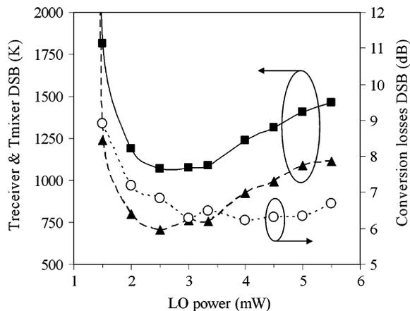
Fig. 4. Measured performance versus LO pump power, at 330 GHz. The top plain curve with filled squares shows the DSB receiver noise temperature, the middle dashed curve with filled triangles shows the mixer DSB noise temperature and the bottom dotted curve with open circles shows the DSB mixer conversion losses. The IF frequency is centered at 1.5 GHz.
