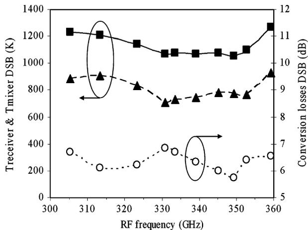
Fig. 3. Measured performance versus RF frequency. The top plain curve with filled squares shows the DSB receiver noise temperature, the middle dashed curve with filled triangles shows the mixer DSB noise temperature and the bottom dotted curve with open circles shows the DSB mixer conversion losses. The IF frequency is centered at 1.5 GHz.
