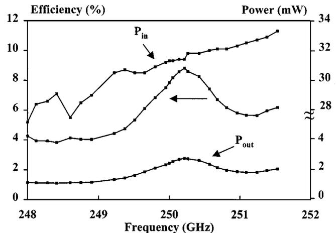
Fig. 8. Input and output power along with conversion efficiency versus frequency. The diode diameter is  $6 \mu\text{m}$ . The number of barriers is four. The input frequencies corresponding to this band are  $82.66$  and  $84$  GHz, respectively.
