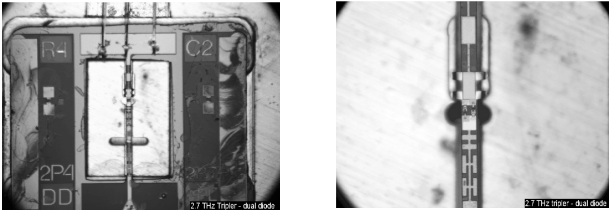
Fig. 3. Left: MOMED tripler shown mounted in waveguide block lower half. Output waveguide is above center, input backshort cavity below center. Right: Blow up showing output waveguide region with mounted antiparallel-pair membrane diodes.
